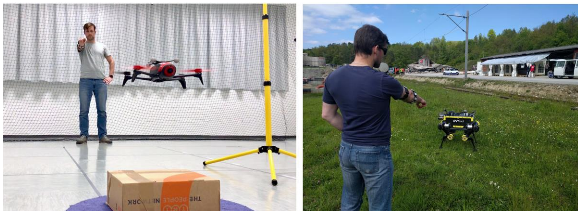
Fig. 14. Human–robot interface in which the operator uses pointing gestures, estimated from sensors worn in armbands, to provide navigation commands to both flying and legged robots
