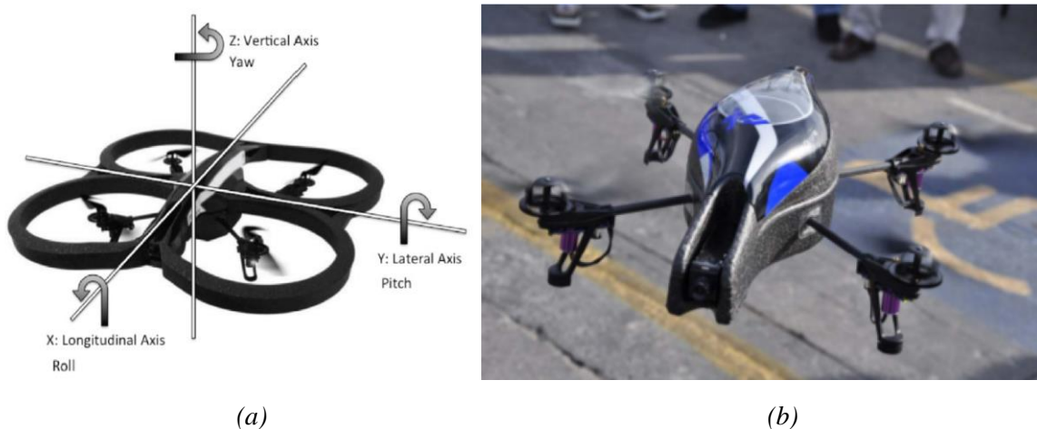
Fig. 21. (a) Movement or principal axis of a drone. The drone is facing the x-axis direction and presents high levels of movement freedom; (b) Picture of the Parrot AR Drone 2.0 [35]
